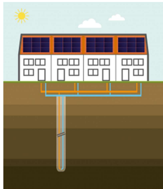
Figure 12: All-electric with collective heat pump network
