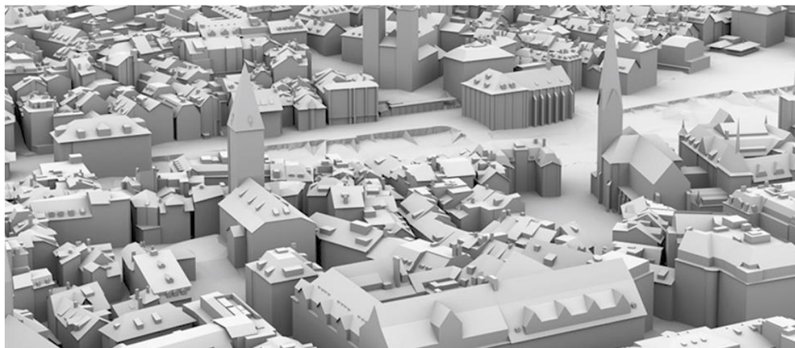
Figure 3 The 3D Spatial model (LoD1, 2 & 3 combined) | Source: Stadt Zürich Geomatik + Vermessung Geodaten (2022)
