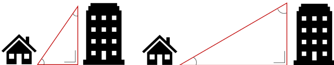
Figure 6: Left: wide building angle as a result of a tall building nearby, right: narrow building angle as distance decays.
