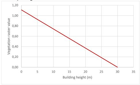
When  $x=0 \rightarrow y = 10/9$ So, the linear function is y = -1/27 x + 10/9
