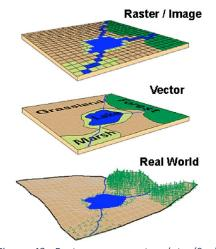
Figure 42: Raster versus vector data (Saab, 2003)
