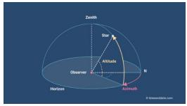
Figure 207: Horizontal coordinate system (Bikos, 2023)
